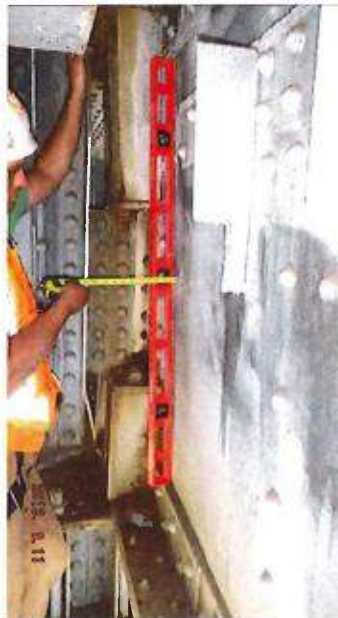
Photograph 4: 1" bowing type deflection damage
